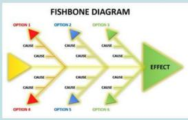
the defect is represented as the head of the fish and the bones represent the major identified root causes. Sub-causes are shown as the ribs of the fish. The technique is widely applied to prevent quality defects. It is a tool that can be used both proactively and reactively.
